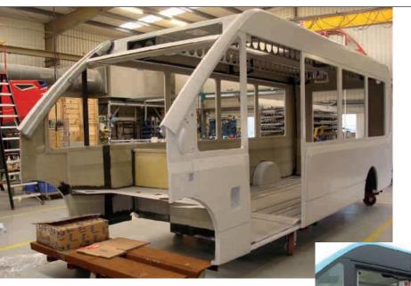
Plastisol's panels are an integral part of the new Bonito. They are combined to form a single body shell to cut weight from the vehicle frame. Nor is it likely to leak – and there's a 10-year warranty on the GRP panels.
